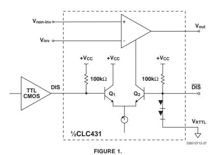
The disable feature of the CLC431 is such that DIS and  $\overline{\text{DIS}}$  have common-mode input voltage ranges of (+V<sub>CC</sub>) to (-V<sub>CC</sub>+3V) and are so guaranteed over the commercial temperature range. Internal clamps (not shown) protect the DIS input from excessive input voltages that could otherwise
